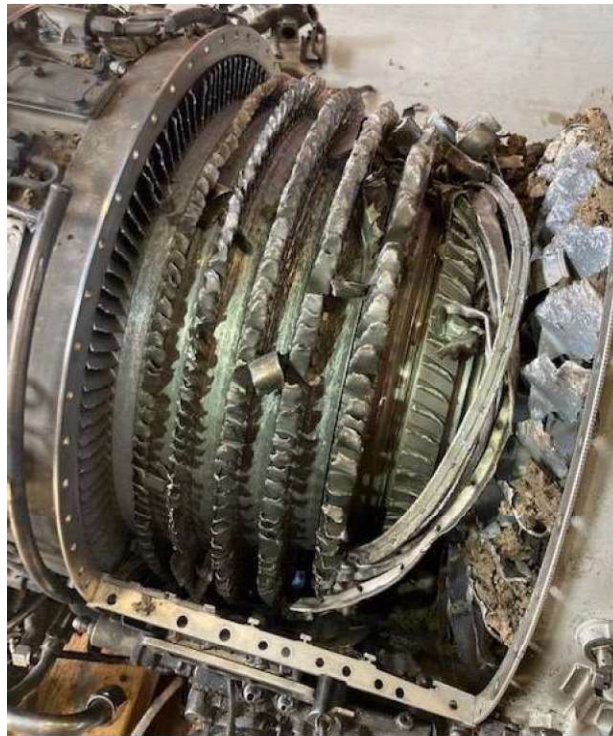
Figure 3 Left engine compressor (Tab J-13)
