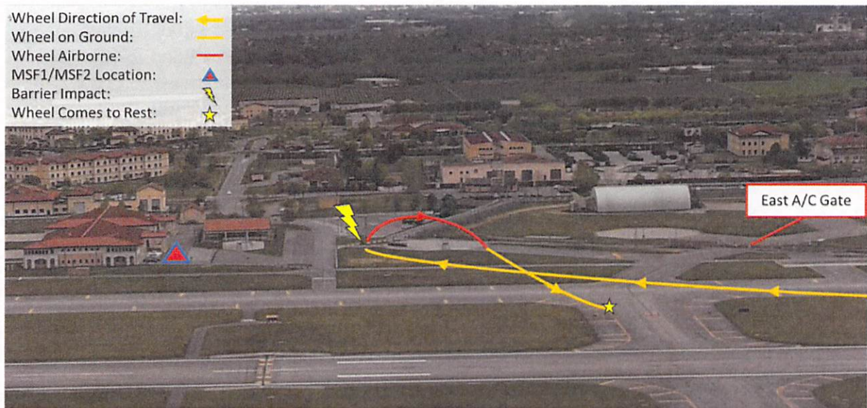
Figure 4 (Tabs R-48 to R-49, R-51, R-53, Z-6, Z-17, and Z-19) Second perspective of the MA's wheel as it bounced around the airfield after dislocating from the MA
