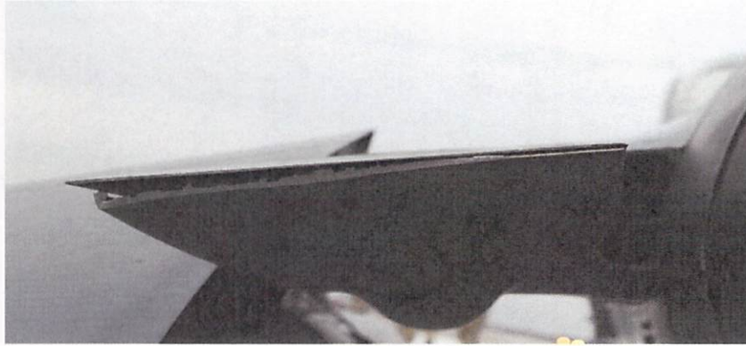
Figure 20 (Tab Z-13) The left speed brake assembly after the mishap
