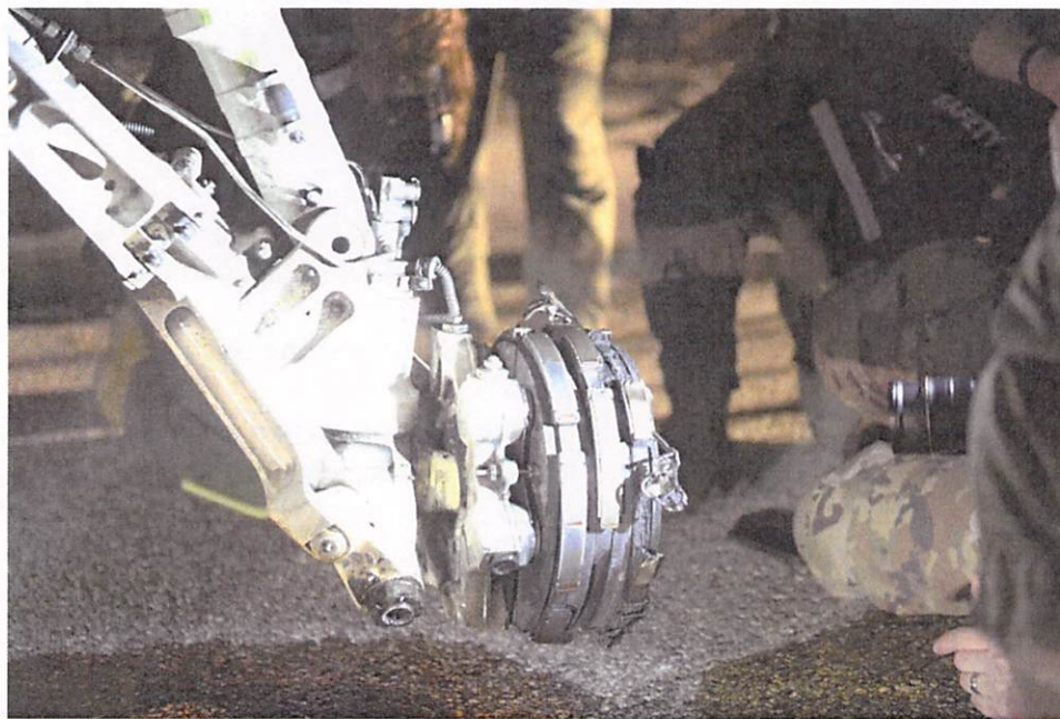
Figure 8 (Tab Z-8) The remaining brake assembly after the MA lost the left wheel
