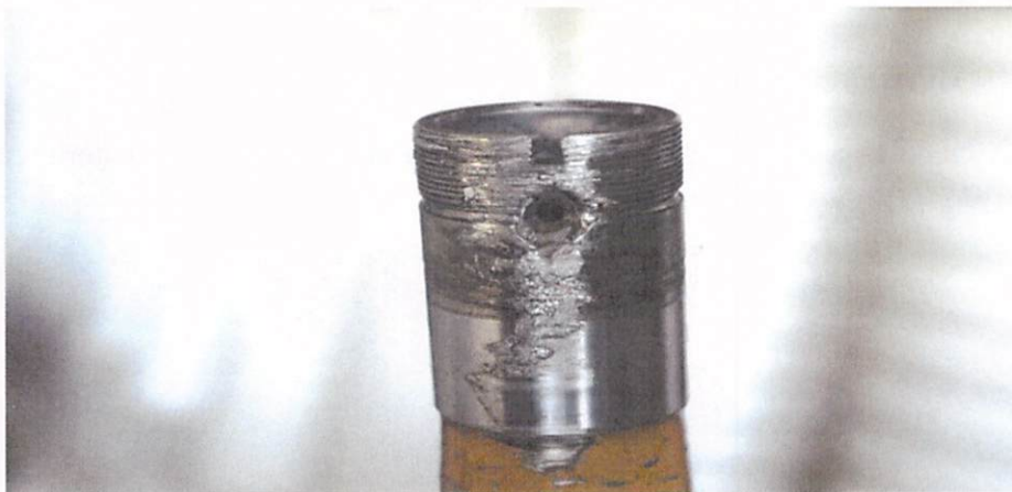
Figure 17 (Tab Z-11) The left MLG axle after the mishap
