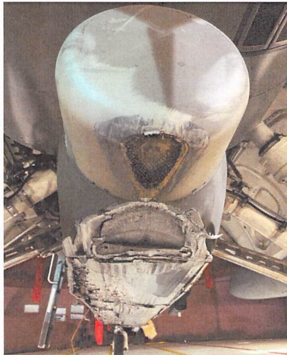
Figure 21 (Tab Z-14) The ECM pod after the mishap
