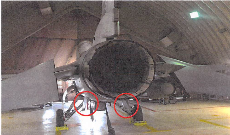
Figure 22 (Tab Z-15) The left and right ventral fins after the mishap
