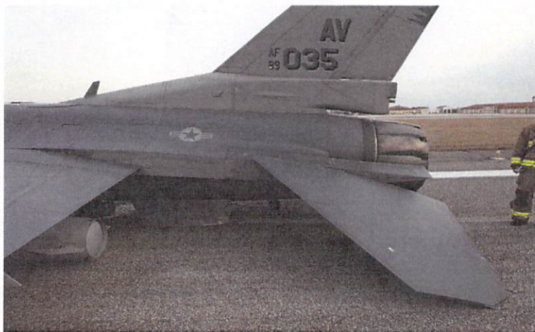
Figure 19 (Tab Z-13) The left horizontal stabilizer after the mishap
