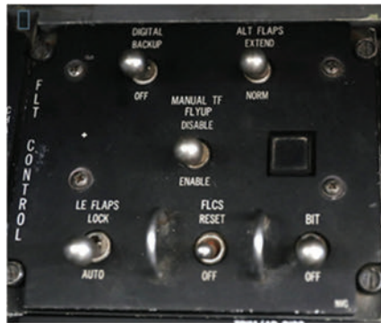
Figure 12: Picture of Flight Control Panel and Proximity of the switches discussed (Tab Z-3)
