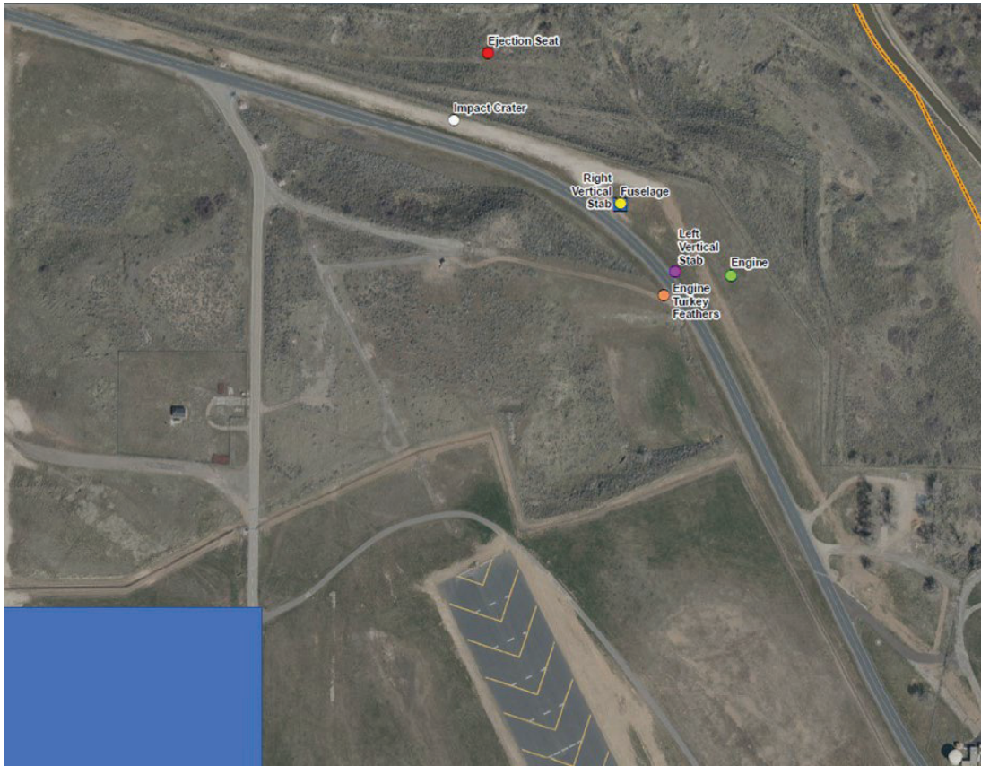
Figure 10: MA debris field on approach end to RWY 14 (Tab S-1.1)
