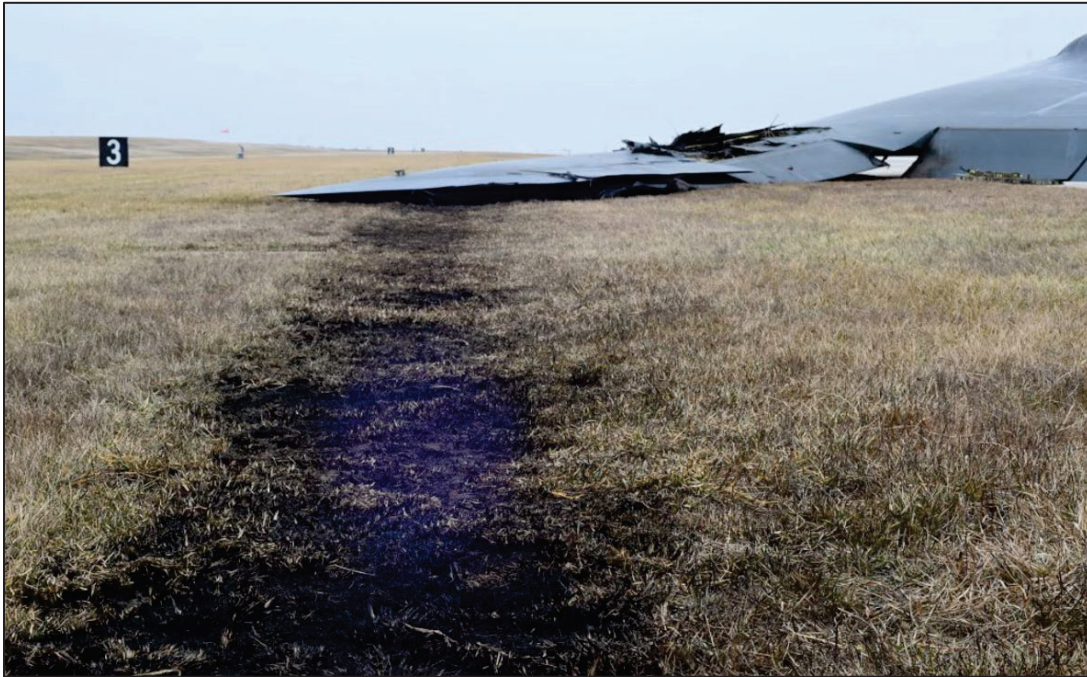
Figure 8: Photograph of Drag and Fire Damage (Tab S-3)
