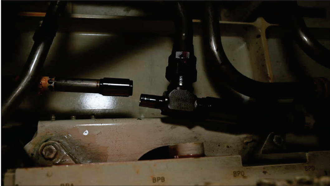
Figure 5: Failed MCC in RMLG Wheel Well (Tab S-14)
