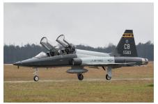
display and an electronic "no drop bomb" scoring system. AETC is the primary user of the T-38C for joint specialized undergraduate pilot training. The instructor and student sit in tandem on rocket-powered ejection seats in a pressurized, air-conditioned cockpit (Tab OO-15).
