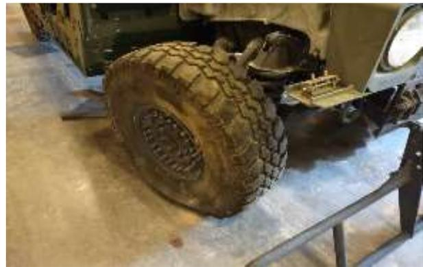
**Figure 8 - Flat Front Right Tire with Broken Bead (Tab Z-6)**
