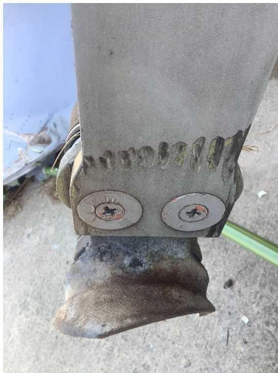
Figure 9: Cable impact marks on hook shank (Tab Z-12)
