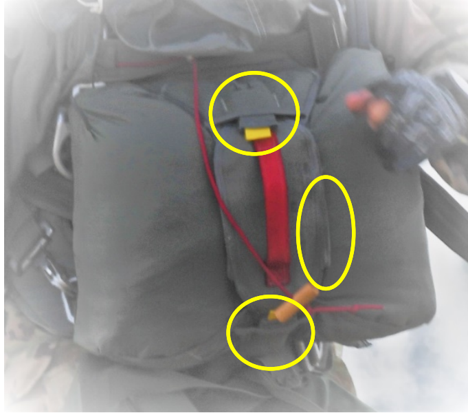
MJM immediately after his first jump with tuck tab inserts Improperly seated and loose left side tuck tab
