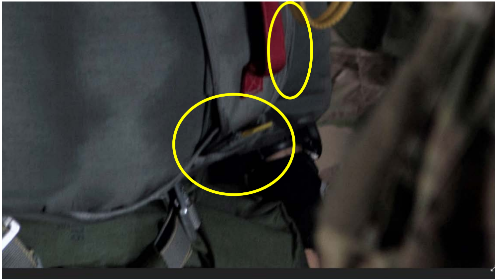
MJM just prior to the mishap with bottom tuck tab insert improperly seated and loose left side tuck tab
