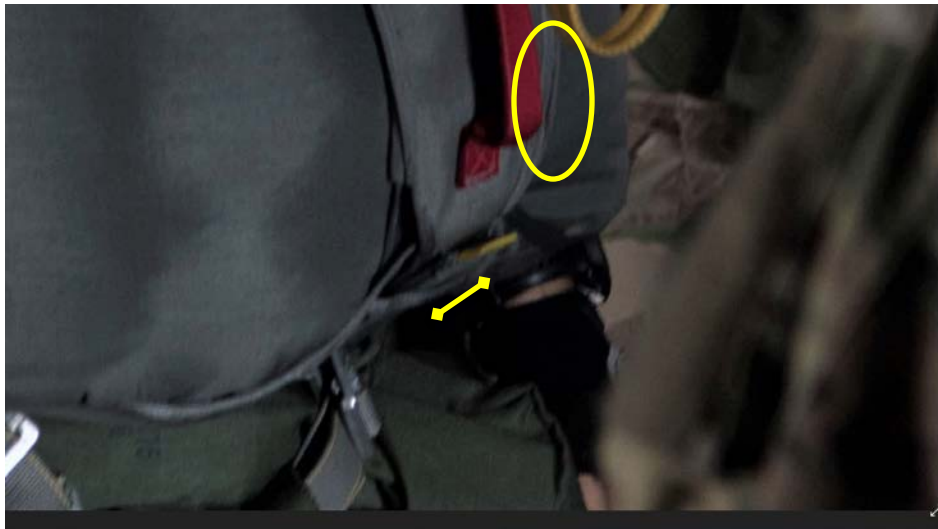
Figure 12. MJM's T-11R parachute just prior to the mishap. The bottom tuck tab insert with approximately one inch between the edge of the pocket and the yellow material and left side tuck tab is loose enough to showing two seams. (Tab Z-49)
