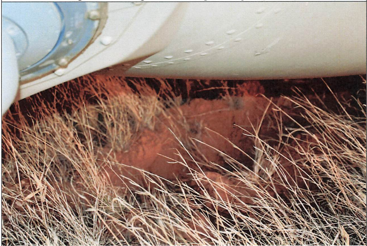
Figure 4-1. MA Right Main Landing Gear Imprint (Tab S-2)
