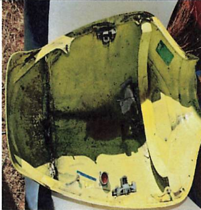
Figure 6.12. Photo of Debris found in LH Centerbody Inlet (Tab S-7)
