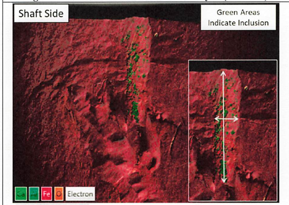
Figure 6-20. Photo of SEM Chemical Analysis (Tab J-55)
