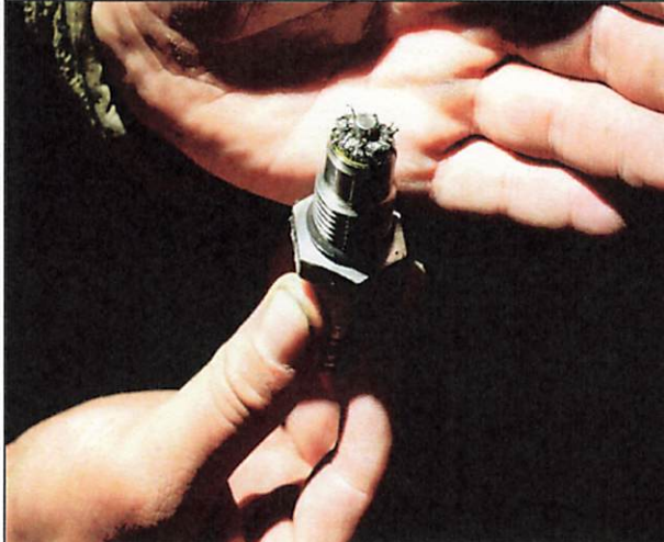
Figure 6.14. Photo of LH PRGB Chip Detector #1 with Debris (Tab S-9)
