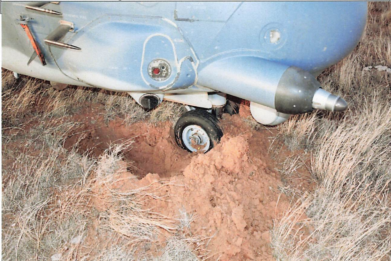
Figure 4-3. MA Nose Gear ditch (Tab S-4)
