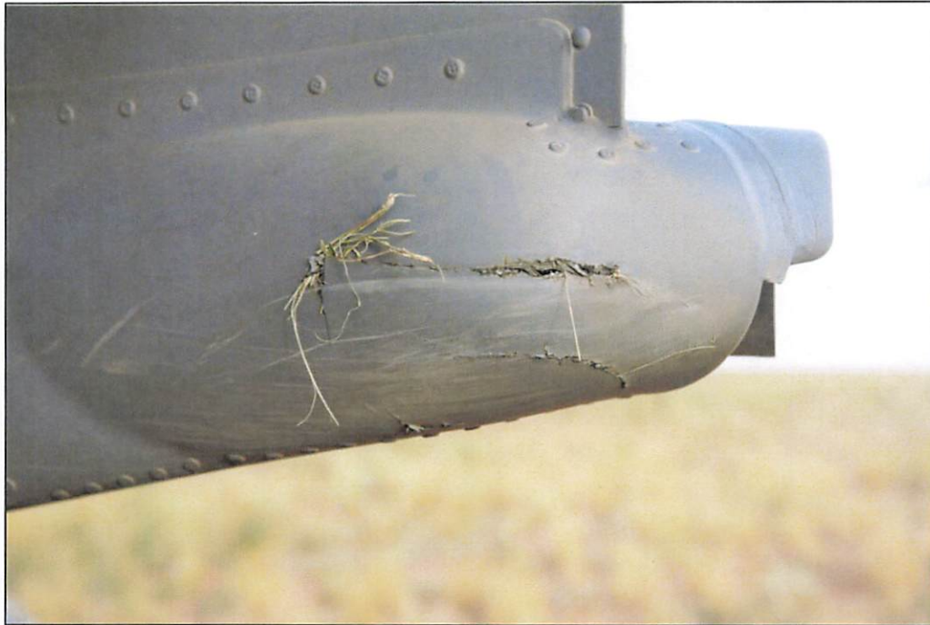
Figure 4-9. MA Damage, Right Vertical Stabilizer (Tab Z-37)
