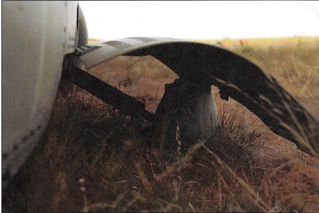
Figure 4-11. MA Damage, Right Gear Door (Tab Z-47)
