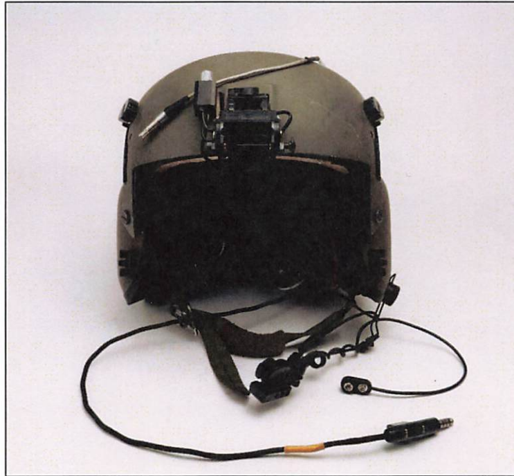
Figure 4-13. MFE1 Helmet with severed NVG cable (Tab EE-3)
