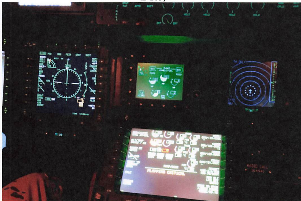
Figure 4-4. Simulator Recreation, FLAPPING CRITICAL posts following impact (Tab Z-103)
