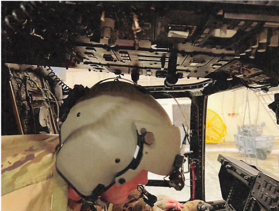
Figure 4-1. FE clearance from ECL while entering cockpit (Tab Z-91)
