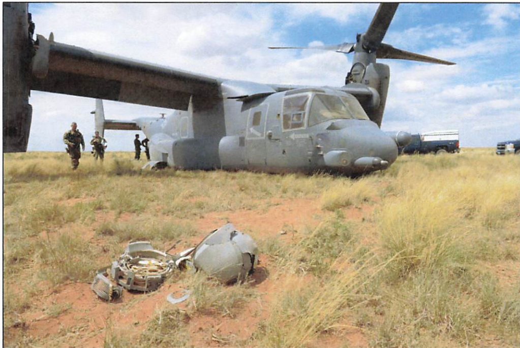
Figure 4-8. MA and FLIR Turret (Tab Z-27)
