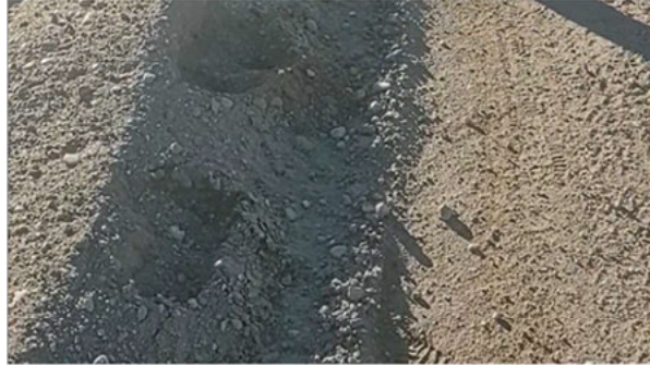
Figure 7-2 (Tab DD-4) 200 lbs Indents in Shoulder of CR 112 6 December 2023
