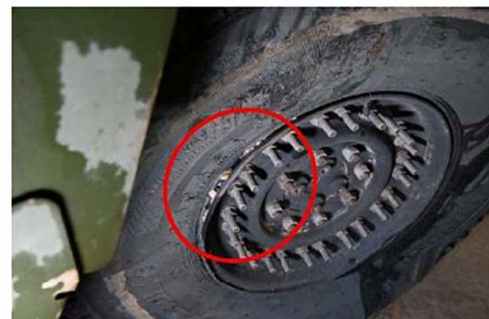
Figure 6-5 (Tab S-186) Broken Bead, Front Right Tire
