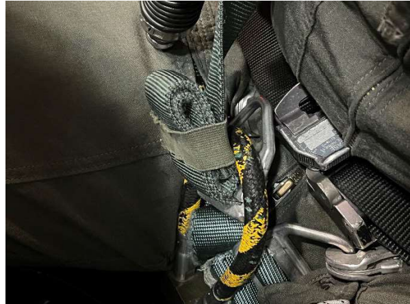
Figure 9: Harness Chest Strap V-Ring in Ejection Seat Control Handle with Pilot Leaning Forward (AIB re-creation) NOTE: the yellow and black handle is the ejection seat control handle. (Tabs LL-2 & MM-2)
