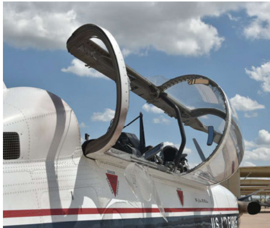
(Figure 11: Mishap Aircraft Fractured Canopy) (Tab Z-6)
