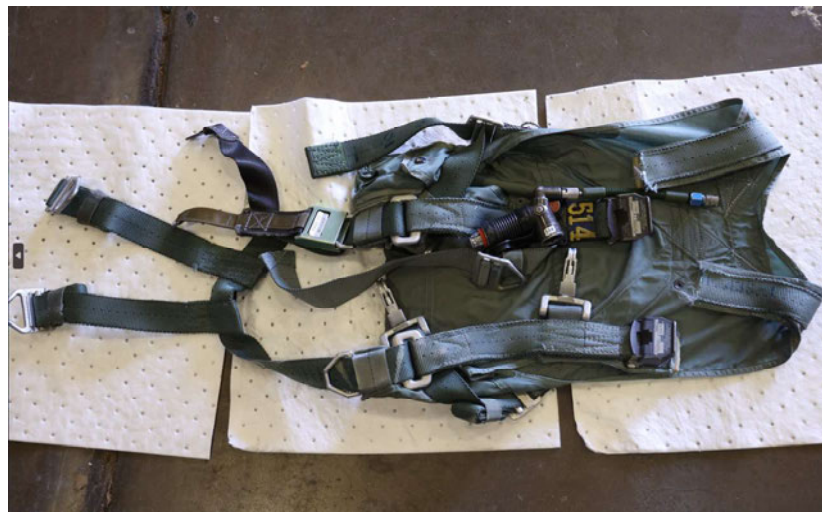
(Figure 19: MIP's PCU-15/P Harness) (Tab Z-13)
