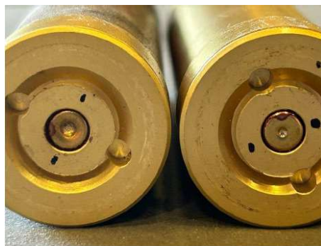
(Figure 12: Mishap Aircraft RCP Seat Initiator Cartridges, Left and Right) (Tab J-3)
