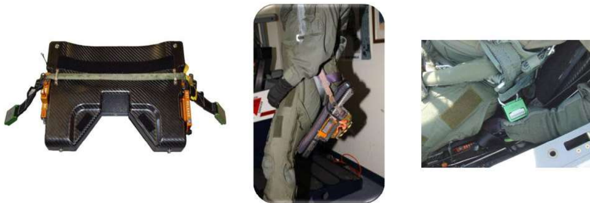
Figure 7: Typical T-6A SSK (left), Typical T-6A SSK Attached to Pilot (center), Typical T-6A SSK Buckled to Pilot Harness (right) (Tabs MM-1 to MM-2)
