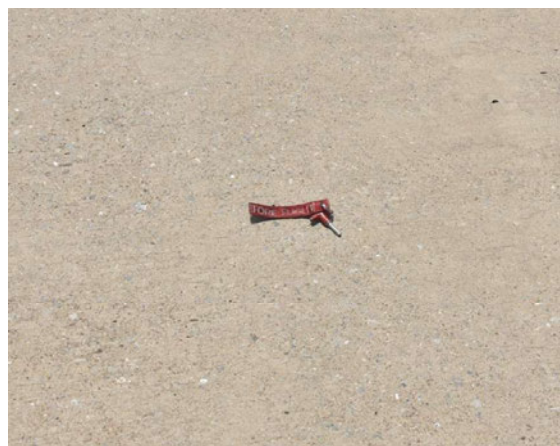
(Figure 14: Mishap Aircraft RCP Seat Safety Pin) (Tab Z-9)
