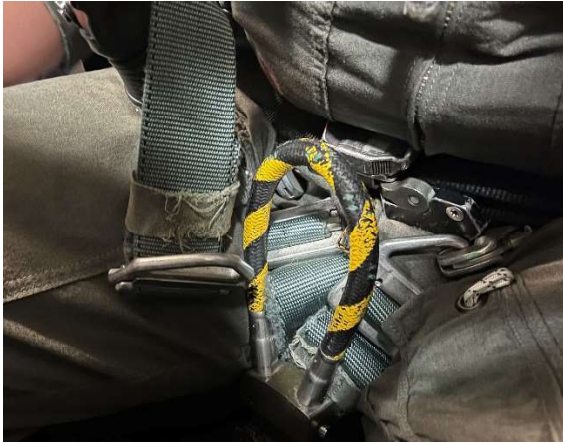
Figure 8: Harness Chest Strap V-Ring Disconnected and Hanging with Pilot Leaning Forward (AIB re-creation) NOTE: the yellow and black handle is the ejection seat control handle. (Tabs LL-2 & MM-2)
