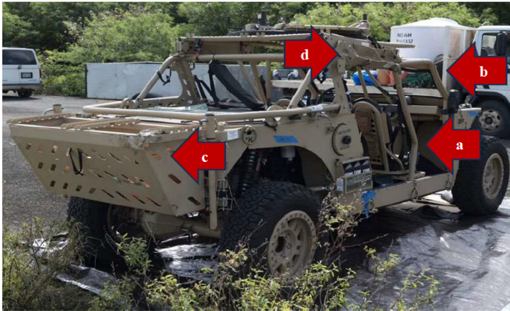
Figure 14: (a) Bent roll cage by passenger seat, (b) Bent windshield frame, (c) Damage to cargo bin on rear passenger side, (d) Crushed bins on passenger side roof (Tab S-142)
