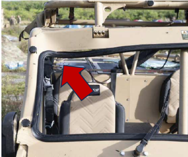
Figure 12: Missing passenger side windshield and bent frame (Tab S-73)
