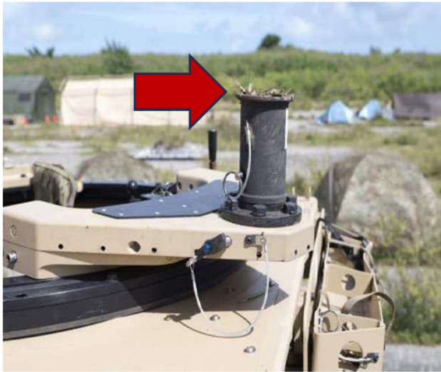
Figure 15: Turret mount packed with dirt and vegetation on roof of the driver side (Tab S-136)
