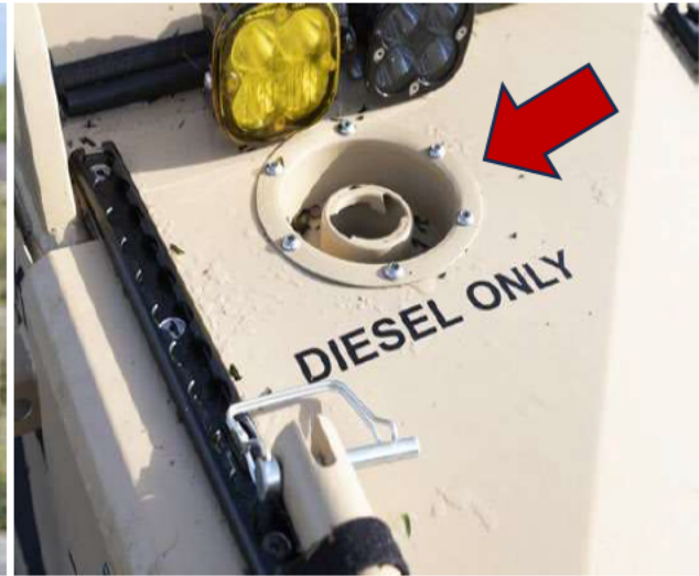
Figure 16: Missing diesel fuel cap on the passenger side hood (Tab S-88)
