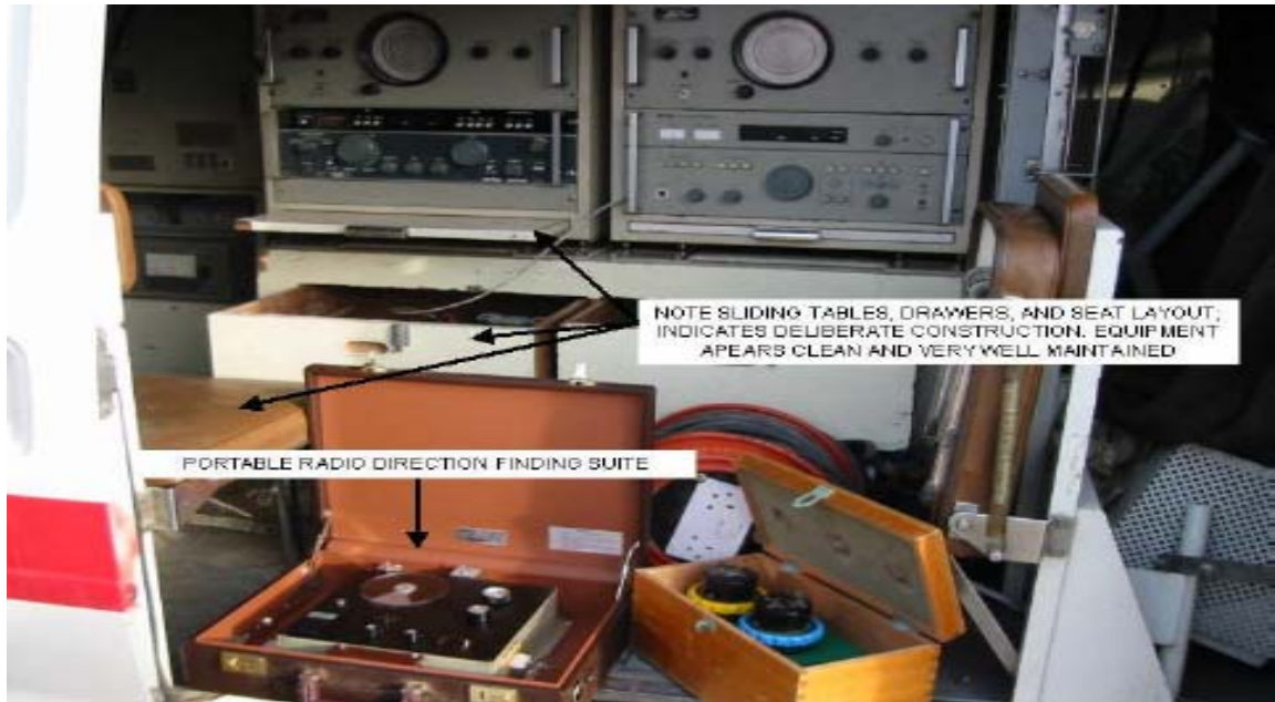
Figure 5—Military Radio Components Inside Iraqi Civilian Ambulance
